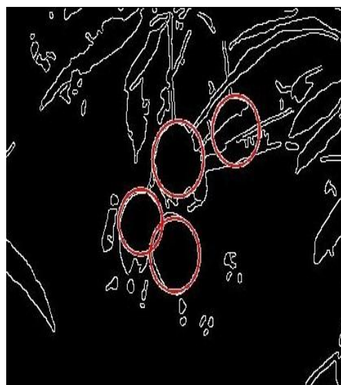
Fig 6: Result of mangoes detection after CHT
